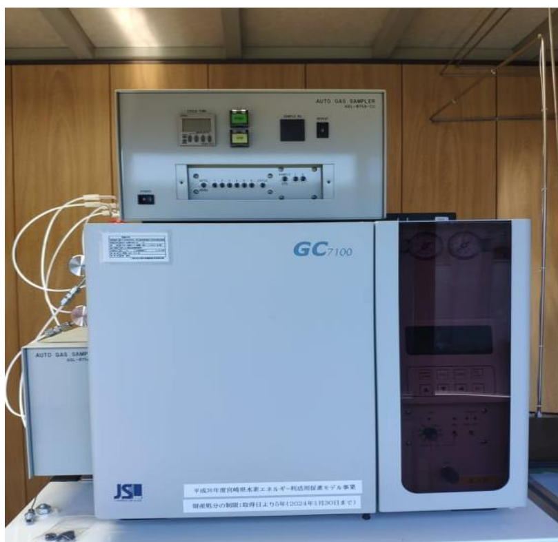
Fig. 3.3 Photograph of gas chromatography, (GC) (J-SCIENCE LAB, GC 7100), installed at the outdoor solar-to-gas conversion field test area of the University of Miyazaki.
