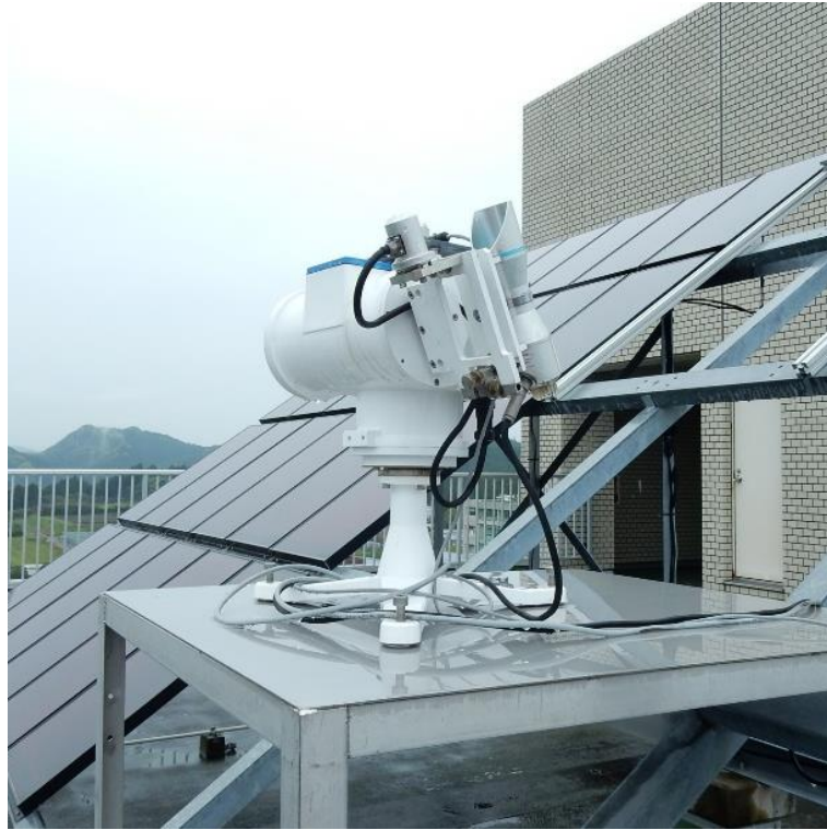
Fig. 2.4. View of pyrheliometer to measure the DNI.
