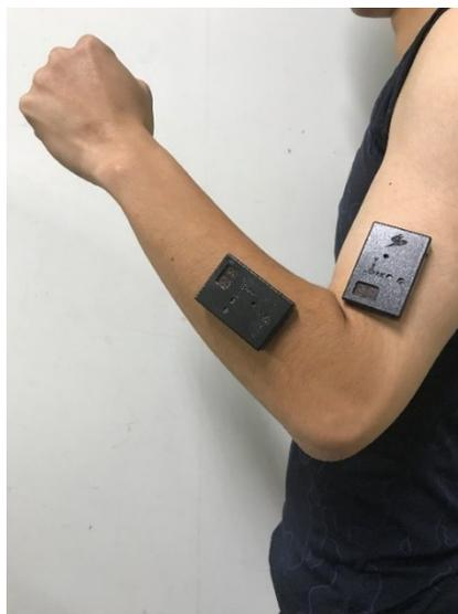
**Figure 2:** Inertial measurement units attached on hand segments
