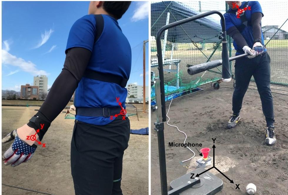
**Figure 22:** positioning of inertial measurement units (IMUs) on body segments
