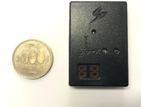
**Figure 13:** Inertial measurement unit used in the current study. 500-yen coin was kept besides for size comparison
