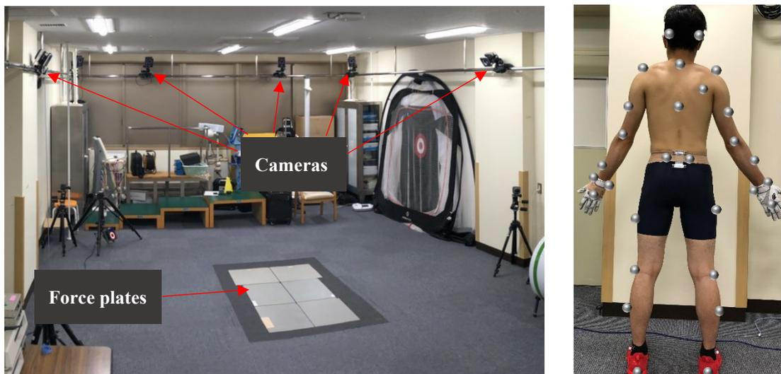
**Figure 1:** Optical motion capture system and reflective marker attachment
