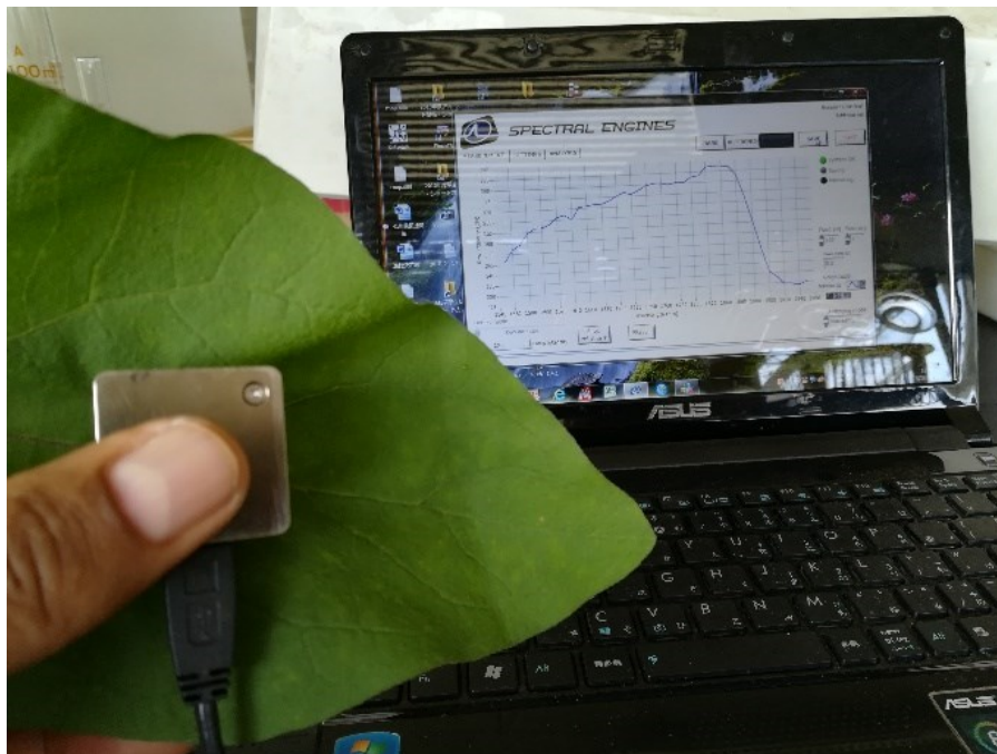
Figure 2.3: Using the hand-held NIRONE Sensor S2.0 to measure leaf reflectance spectra
