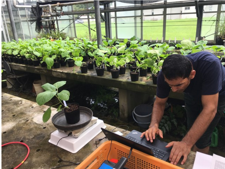
Figure 3.1: Pot gravimetric measurement using a fine-scale electronic balance
