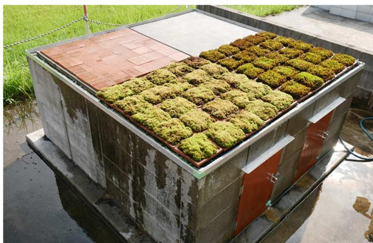
Fig. 4.24. The test structure with moss-covered and ceramic samples.
