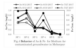
1) Raw water tank (SP-1~SP-2): The concentration of arsenic and iron increase at SP-2, which means the happening of coprecipitated material of Fe with As at the bottom of raw water tank.
