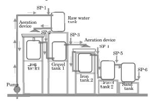
Fig.1 Schematic diagram of prototype Multi-GSF for high As-contaminated groundwater (As  $\ge$  1.0mg/L)
