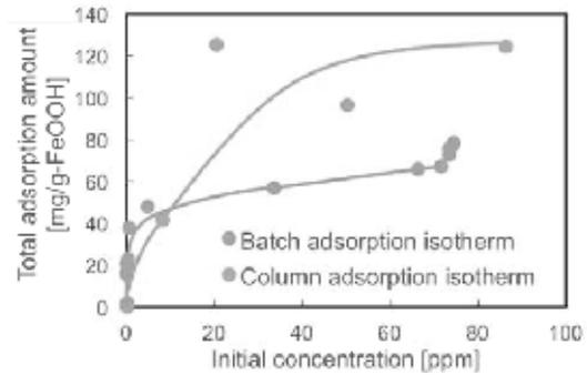
Fig. 3 Relationship between total adsorption amount and initial concentration of As(V).
