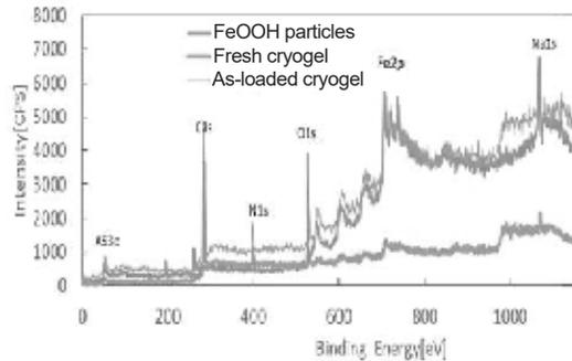
Fig. 4 XPS wide-scan spectra of FeOOH particles and the adsorbents before and after As(V) adsorption.
