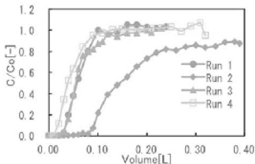
Fig. 2 Break through curves of the column adsorption of As(V) under the condition in Tabel 1.
