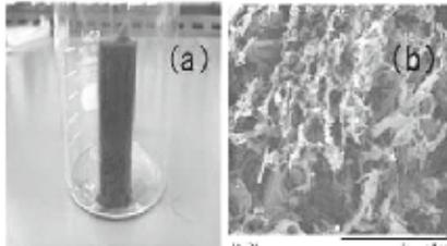
Fig. 1 Observation of the cryogel containing FeOOH particles. (a) external appearance, (b) surface by SEM.
