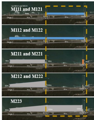
Figure 4.26 Sand volume change at compartment 2 (between Groin 2 and Groin 3) in the nourished area
