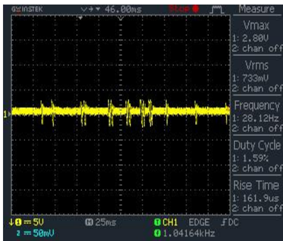
Fig.5. Typical waveform as copper sparking gap
