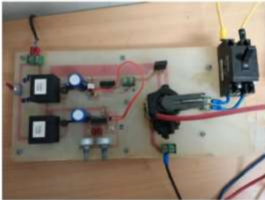
Fig 3. complete circuit of the thin film fabrication with spark technique
