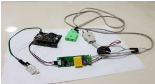
Fig. 1. Assembling Arduino NodeMCU V.3 with PZEM-004T and DHT22
