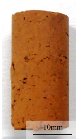
Figure 2.5 Appearance of the compression test specimen
