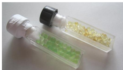
Fig. 4 HDI beads under dry (left, green) and wet (right, orange) conditions in a quartz cell
