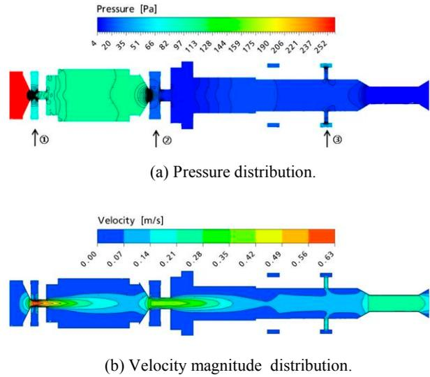
Fig. 7. Computational results in middle section along the oil forming nozzle.
