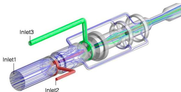
Fig. 10. Streamlines of multi-stage nozzle.
