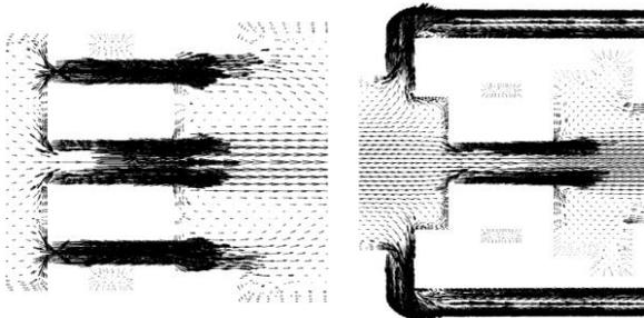
Fig. 6. Velocity vectors around oil forming chamber
