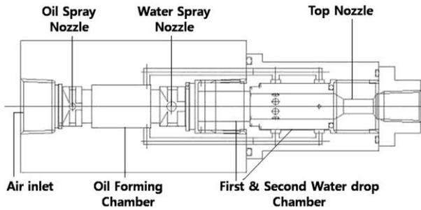
Fig. 1. Schematic diagram of multi-stage nozzle .
