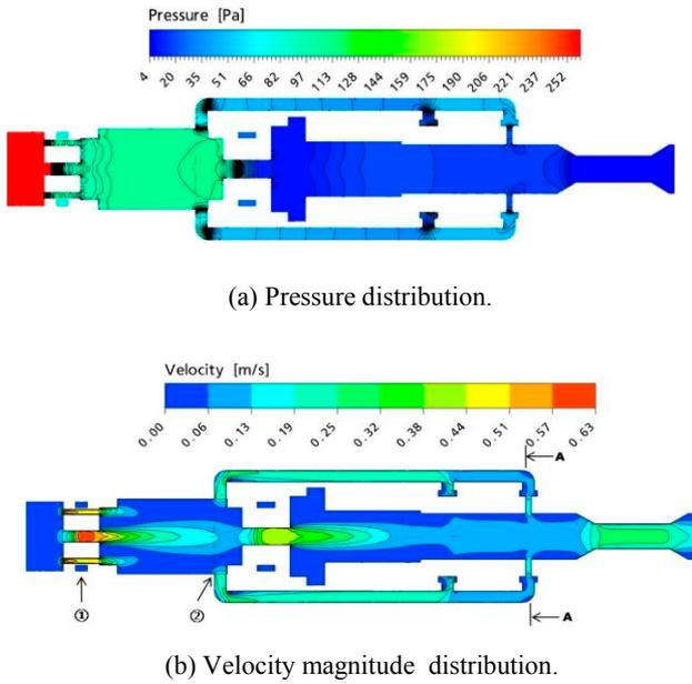
Fig. 5. Computational results in the middle section along the water spray nozzle.
