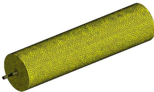
Fig. 2. Computational grid of top nozzle.
