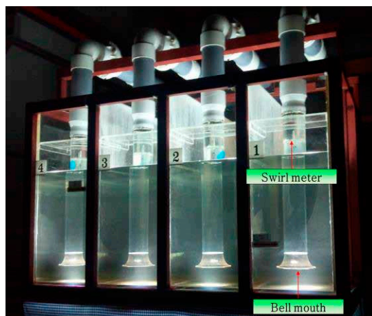
Fig. 2. Bell mouth chamber and observation window.
