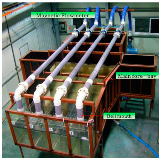
Fig. 1. Test model sump with four water intakes.
