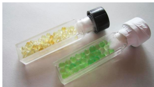
Fig. 4 HDI beads under wet (left) and dry (right) conditions in a quartz cell.
