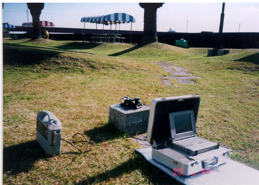
Fig.2.3-1. Microtremor observation unit and pick-ups.
