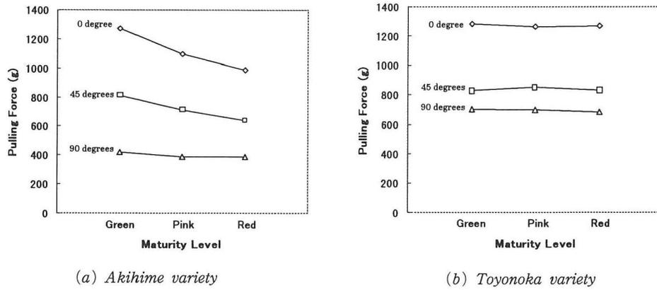
Fig. 5. The average pulling forces for three maturity levels of *Akihime* and *Toyonoka* strawberries at three pulling angles.
