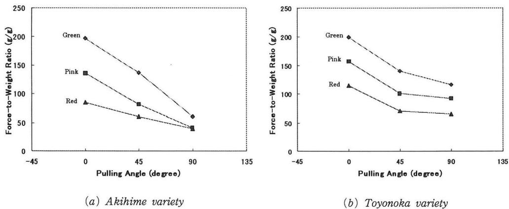
Fig. 7. The average force-to-weight ratio values for three maturity levels of *Akihime* and *Toyonoka* strawberries at three pulling angles.
