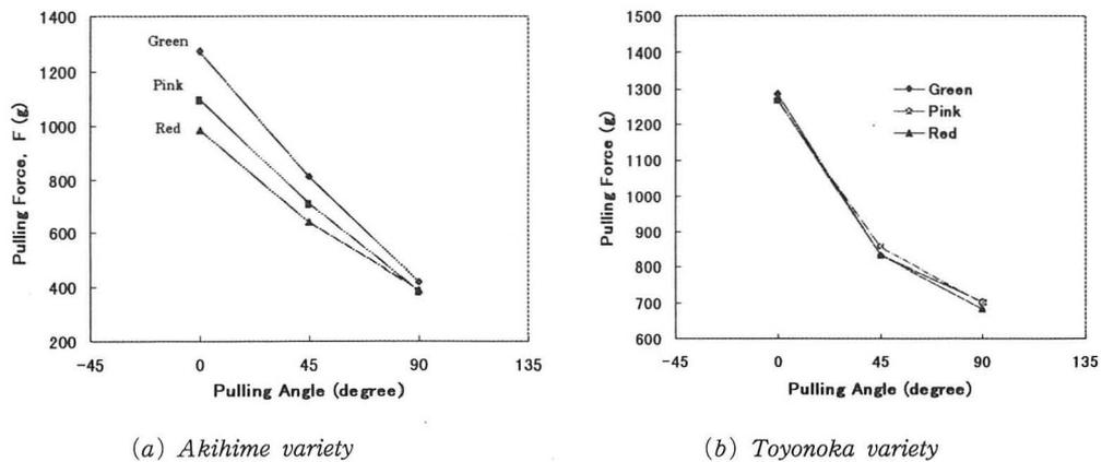
**Fig. 4.** The average pulling forces for three maturity levels of *Akihime* and *Toyonoka* strawberries at three pulling angles.
