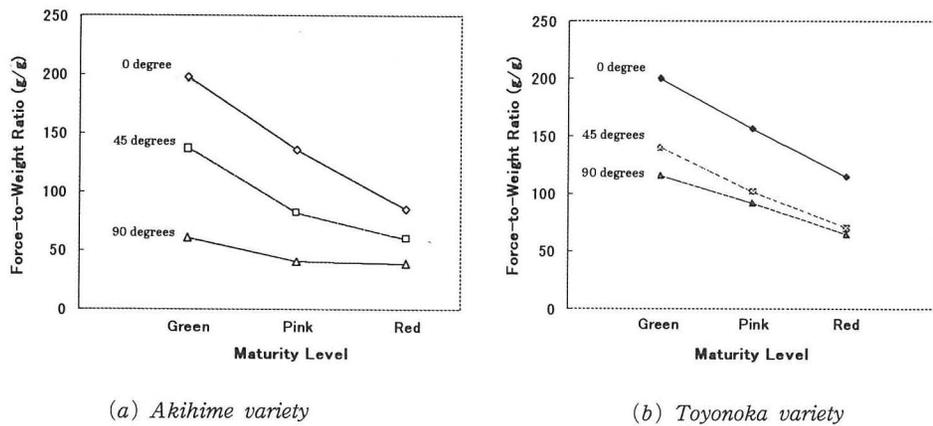
Fig. 6. The average force-to-weight ratio values for three maturity levels of *Akihime* and *Toyonoka* strawberries at three pulling angles.
