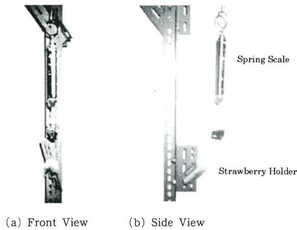
Fig. 2. Setup used in the strawberry pulling tests.
