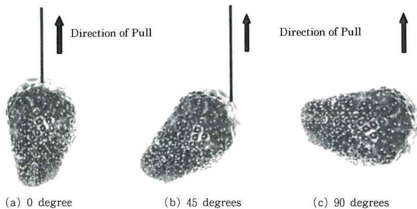
Fig. 3. The three pulling angles used in the experiment.
