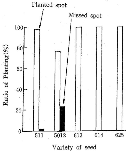
Fig 11. Ratio of Planting on Corn Planter of Inclined-Plate Type
