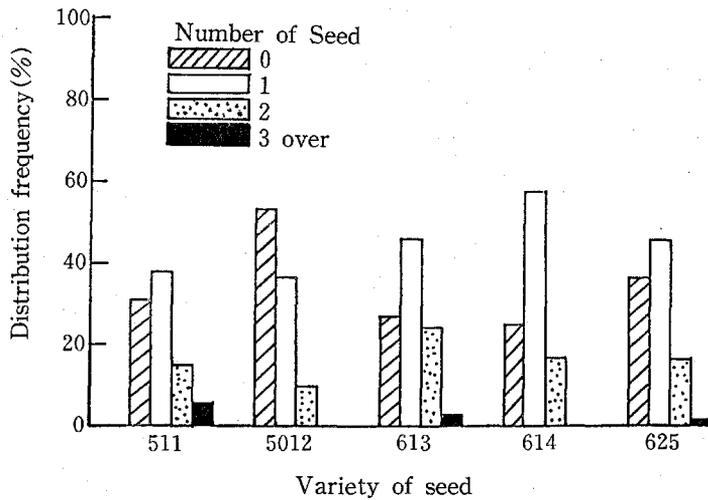
Fig. 8. Distribution Frequency of Metering Seed
