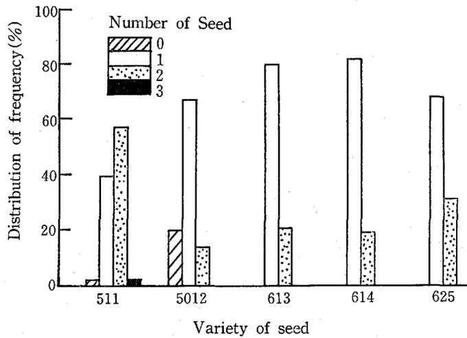
Fig 12. Distribution Frequency of Metering Seed on Corn Planter of Inclined-Plate Type
