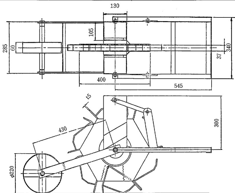
Fig. 4. Reconstructed Corn Planter of Rolling Injection Type for Testing
