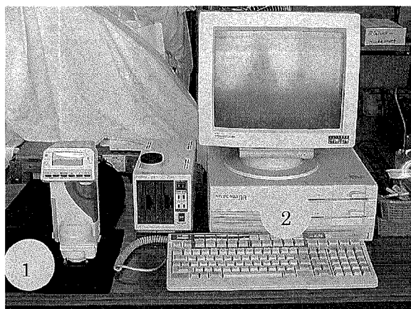
1. Spectrophotometer Minolta (CM-508i Series) 2. Computer (NEC-PC9800)
