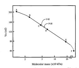
**Fig. 1.** Determination of molecular masses of inulinases P-II and P-III from *A. niger* 12 on a Sephadex G-200 gel-filtration column.
