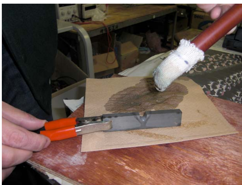
Fig. 5.7 Electrolytic polishing device and method
