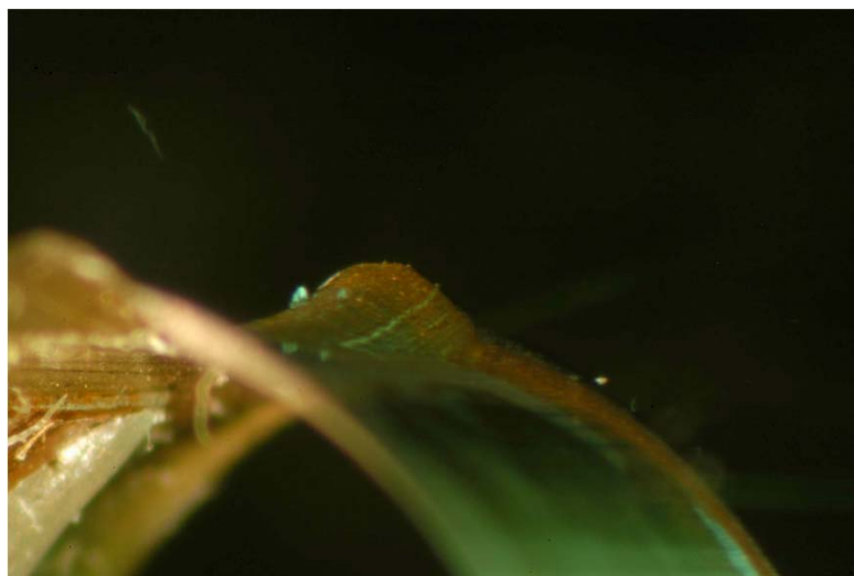
Fig. 1.6 A small crack on the notch surface of an acrylic test piece
