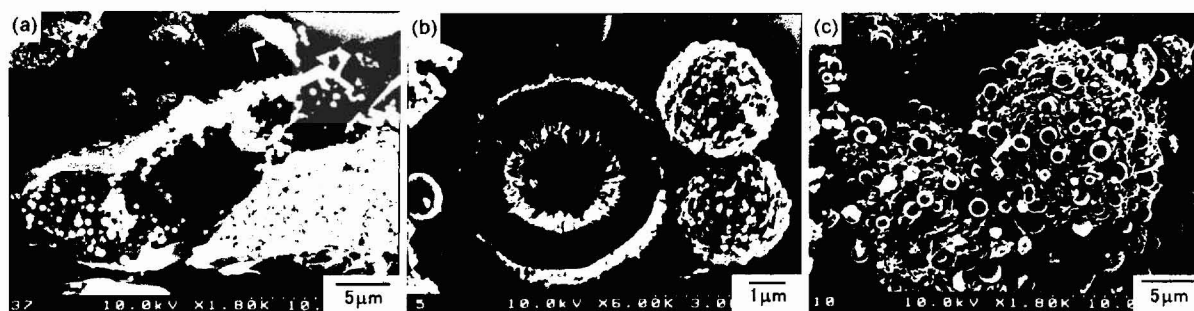
Fig.7 SEM images of the final products derived from \text{SnCl}_4 /hexylamine/ \text{H}_2\text{O} systems at molar ratio of (a)1:2:60, (b)1:5:60, and (c)1:10:60.
