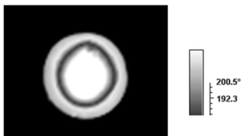
Fig.10 Temperature distribution of bottom face.
