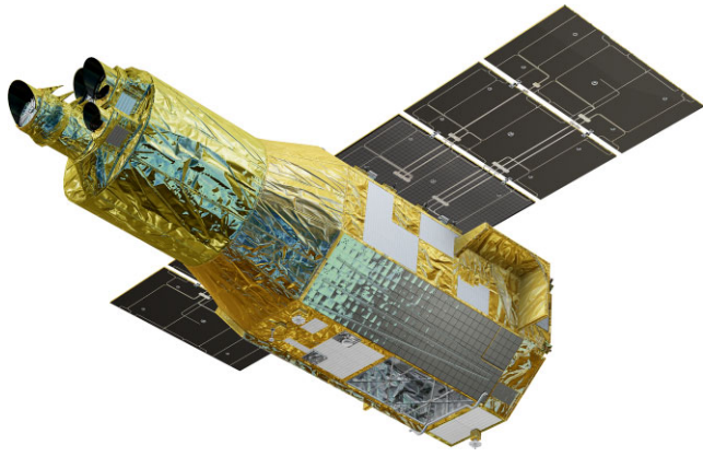
Fig. 1. Outlook of XRISM and onboard mission instruments. Two X-ray mirror assemblies and three star tracker units are equipped on the top plate on the upper left. The solar panel arrays are the dark wing-shaped structures in the center. Credit: JAXA.
