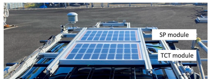
Fig. 2. Experimental setup on the car roof, featuring SP and TCT PV modules installed horizontally alongside a pyranometer. The system also incorporates a commercial PV module.
