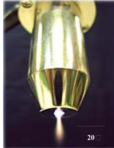
Fig. 3. Photograph of high-frequency dc pulse discharge plasma jet.
