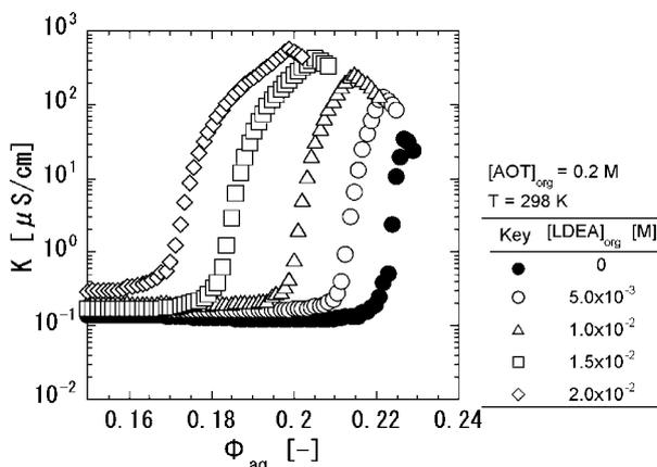
**Fig. 4.** Effect of the LDEA concentration on the percolation process of the mixed reverse micellar solution of AOT and LDEA.
