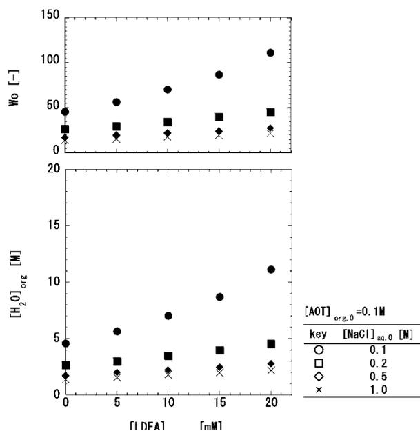
**Fig. 2.** Effect of LDEA concentration on the water extraction into the reverse micellar phase at various NaCl concentration in the aqueous phase and 0.1 M AOT in the organic phase
