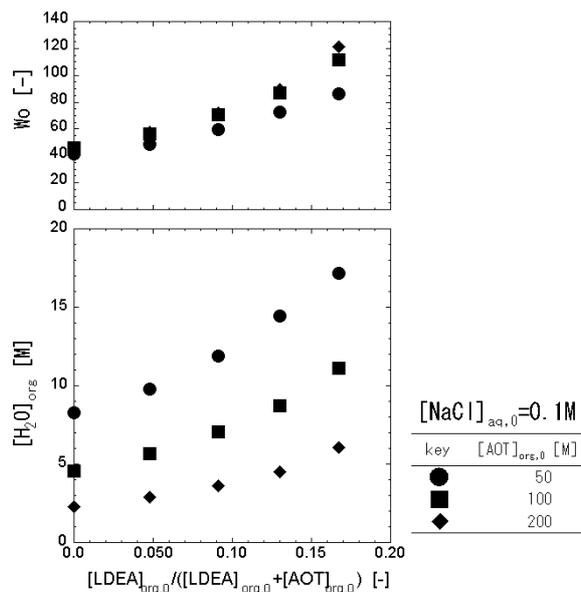
**Fig. 3.** Effect of the molar ratio of LDEA to total surfactant concentration in the organic phase on the water extraction
