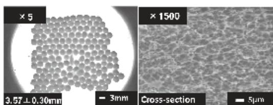
Fig. 1 Observation of the microcapsules containing LIX84-I by digital microscope (left) and its cross-section by SEM (right).
