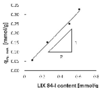
Fig. 3 Effect of the LIX84-I content on the maximum extraction amount  $q_{eq,max}$ .
