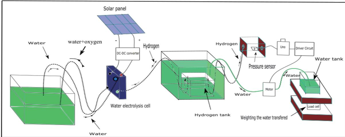
Fig 1. The hydrogen production system overall diagram
