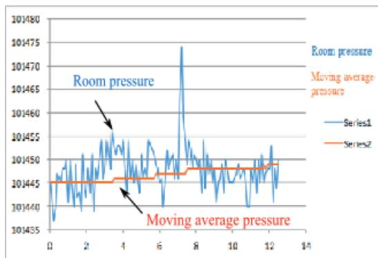
Fig 3. Room pressure sensor data
